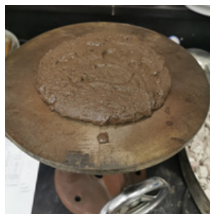
Figure 2: Flow table test of GPM
