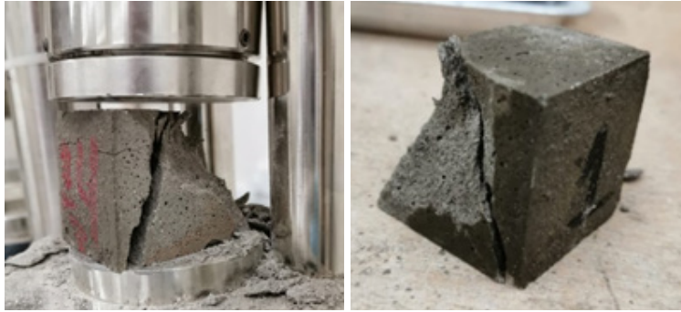
Figure 1: Compressive strength of GPM cube.
