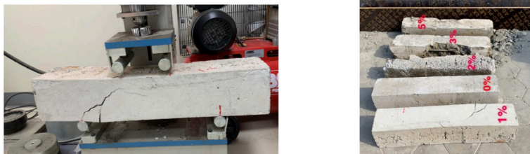
Figure 9: Concrete beam samples during and after test
