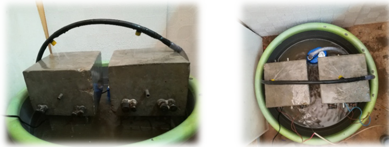
Figure 6: Test setup for beams group.
