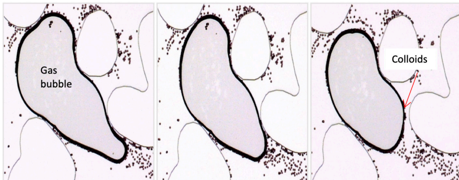
Figure 7: Snapshots of dissolution of Gas bubble ( \text{CO}_2 ) during imbibition at higher ionic strength. The excess particles on GWI reattach on SWI (bottom of the micromodel), as the adhesive forces were greater
