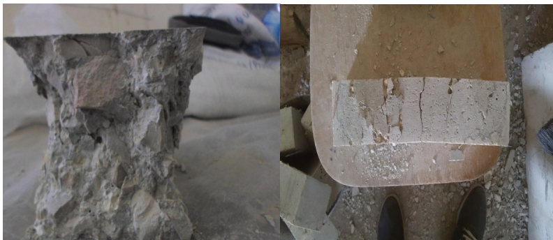
After compressive test
