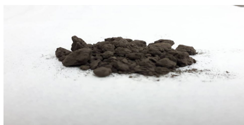
Figure 2: Grinded steel slag sample
