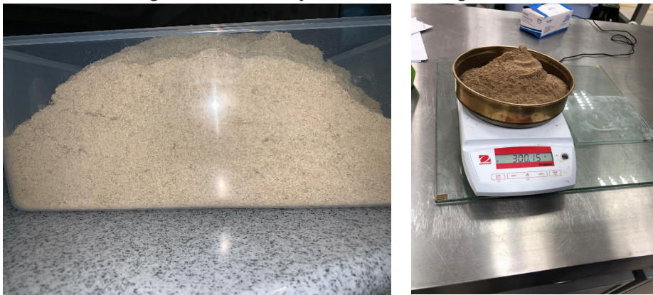
Figure 3: (a) PTF powder, (b) 300 gr of PTF powder extracted from 1.7 kg of PTF fiber
