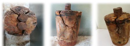
Figure 3: Crack pattern at lapped spliced joint in cylinder samples in: a) c/d = 2.6; b) c/d = 1.5.
