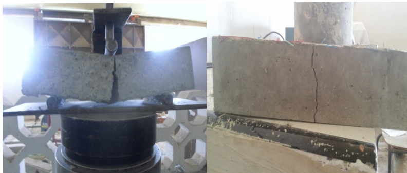
After flexural test
