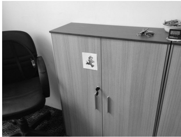
Fig. 5. A visual AR marker/sticker with an image of Mario computer game character attached to a real-world object.
