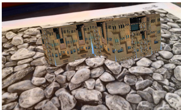
Fig. 2. The 3D model of the building using AR read tag based on image.
