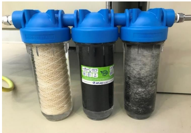
Figure 3-6: Triple filtration stage for tap water by ATLAS FILTRI.
