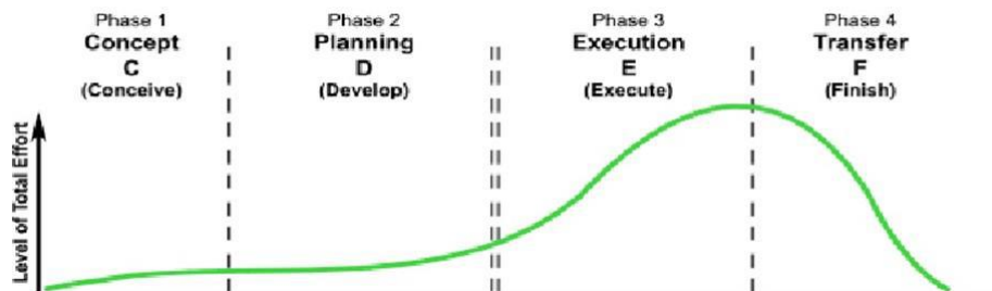
Figure 1. Life Cycle Of A Construction Project
