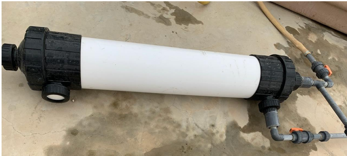
Figure 3: Tangential flow filtration (TFF) unit
