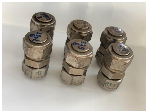
Figure 4: 10 mL high-pressure Swagelok fitting type reactors
