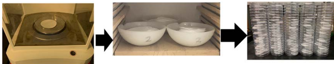
Figure 5. Preparation of the Whatman GF/F filters by weighing (left), ashing (middle), then labeling and storage of the filters (right).
