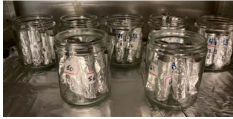
Figure 7. SPM on GF/F membrane filter. Sample were dried at 60 °C, placed in labeled, aluminum foil tubes in a pre-combusted glass jars.
