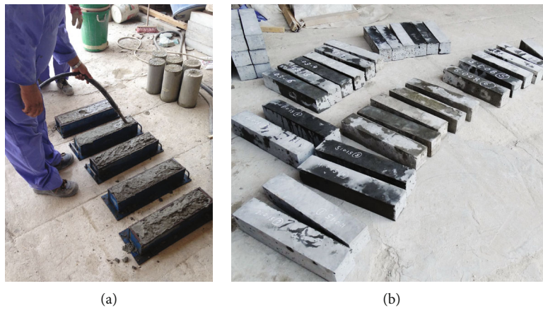
FIGURE 2: (a) Specimen compaction using a vibrator. (b) Specimen after 28 days of curing.
