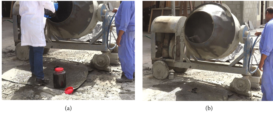
FIGURE 1: (a) Combined CNT solution. (b) Concrete CNT mixing.
