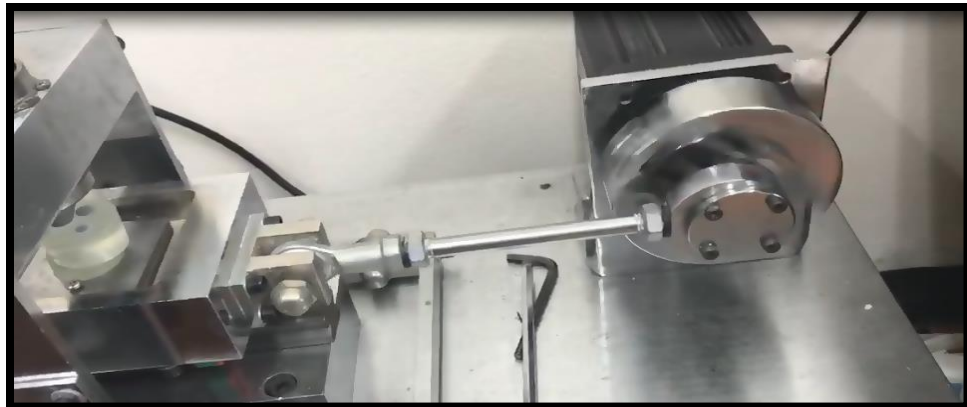
Figure 9.9. Reciprocating wear test machine.
