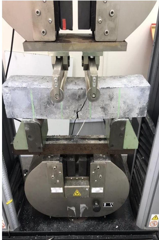
Figure 11. Flexural Tensile Strength Test for Prism Specimen
