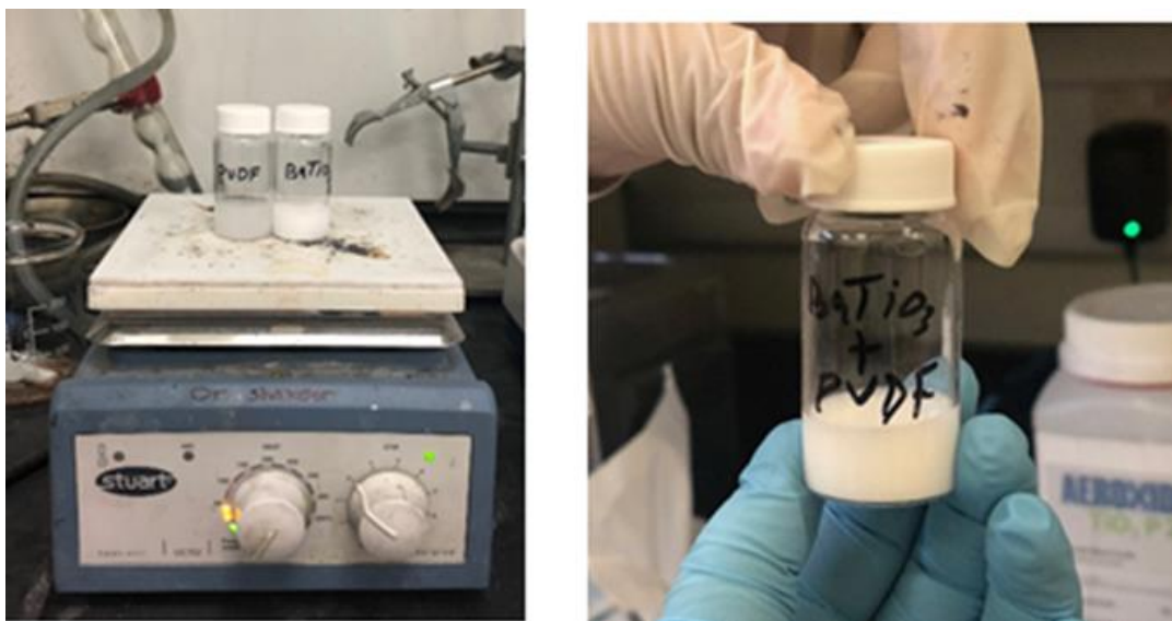
Figure 3-8. Image of magnetic stirring of polymer and nanoparticles on a hot plate.
