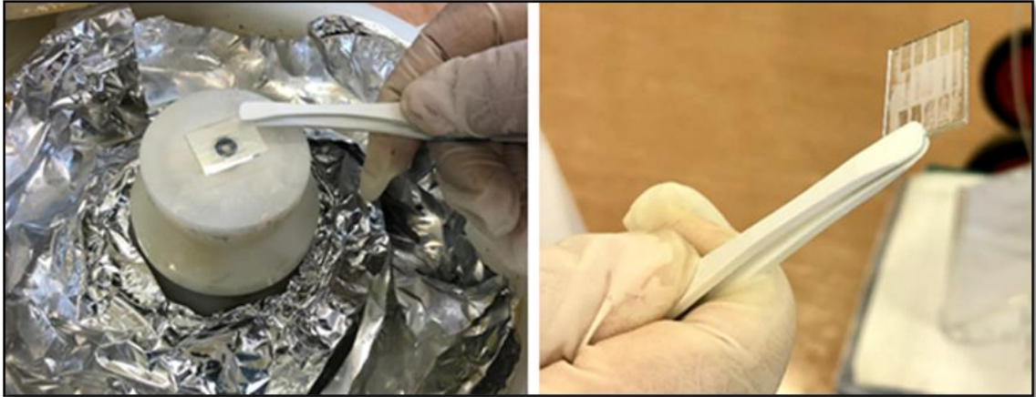
Figure 3-9. Image of Spin coating of polymeric film on the ITO electrode.
