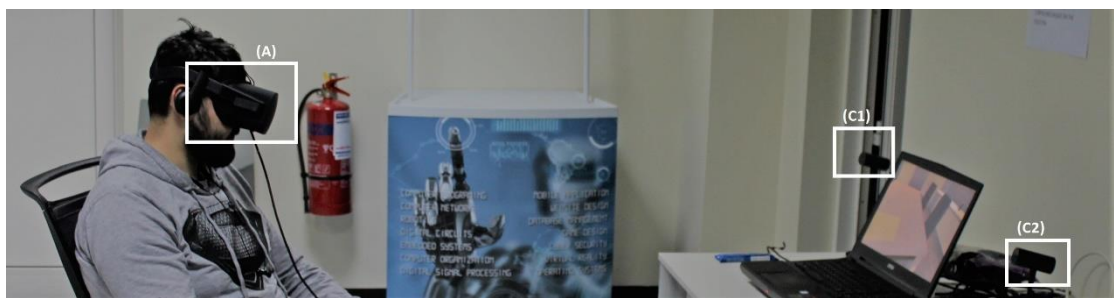
Figure 7. Passive Interaction (A) Oculus Rift CV1 HMD (C1 and C2) Left and Right Sensors
