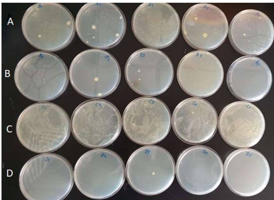
Figure 24. Nutrient agar plates showing the total aerobic bacterial growth of 100 \mu l of the 25ml of sterile distilled water used to wash the surfaces of different strawberry samples used in taking the first reading. Plated are given the names of the treatment with the number of the replicate (1 to 5) (A: negative control; B: sprayed with 8mg/ml PJ-WS-LE extracts; C: coated with 1% chitosan; D: coated with 8mg/ml PJ-WS-LE extracts embedded in 1% chitosan).
