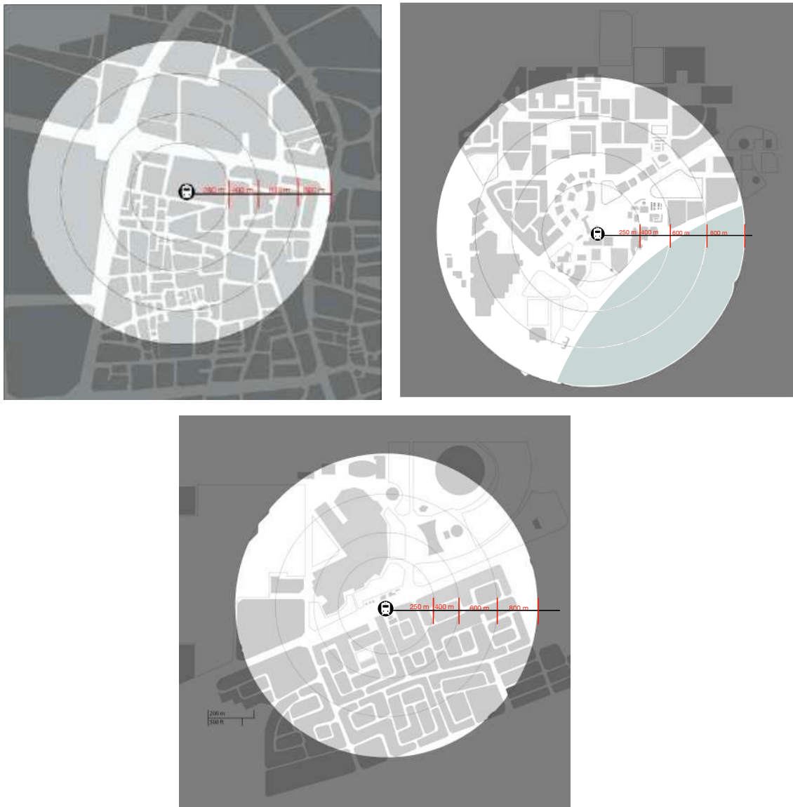
Figure 42. Pedestrian shed for a 5-minute walk (250-400 m) from (top left) Hamad Hospital Station, (top right) West Bay Station, and (bottom) Al Aziziyah Station.
