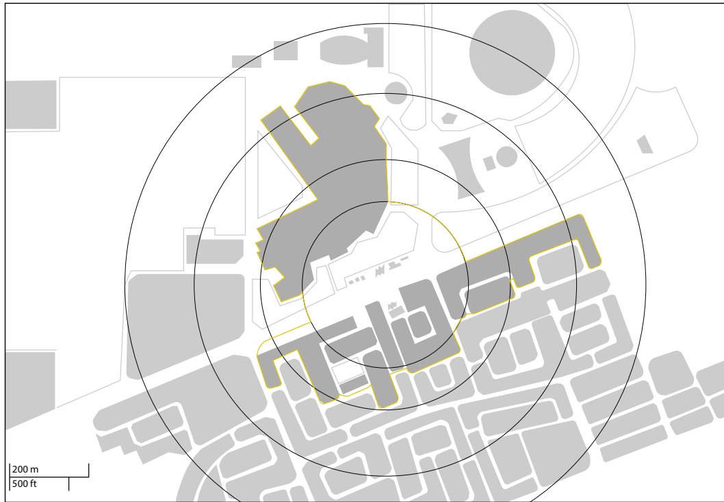
Figure 40. The premises of 250 m radius to calculate the average block size around Al Aziziyah Station and the defined polygon.
