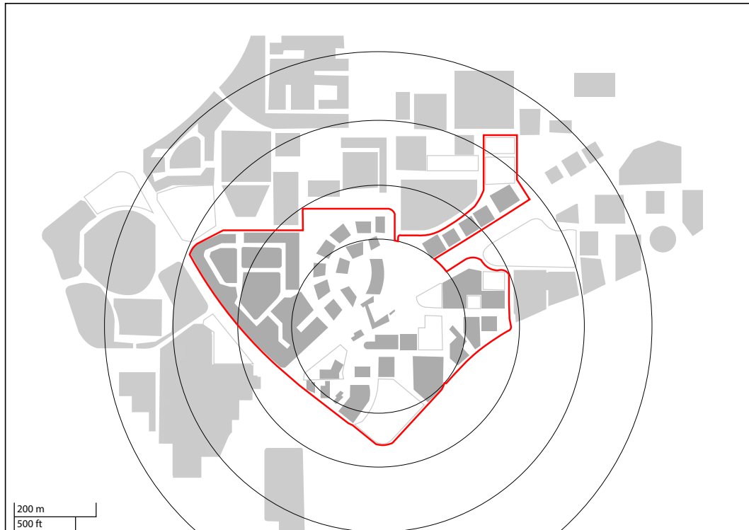
Figure 39. The premises of 250 m radius to calculate average block size around West Bay Station and the defined polygon.
