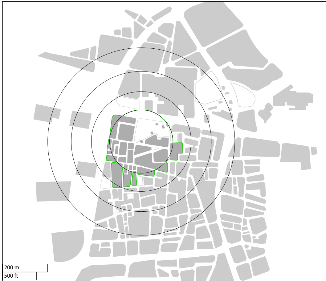
Figure 38. The premises of 250 m radius to calculate average block size around Hamad Hospital Station and the defined polygon.
