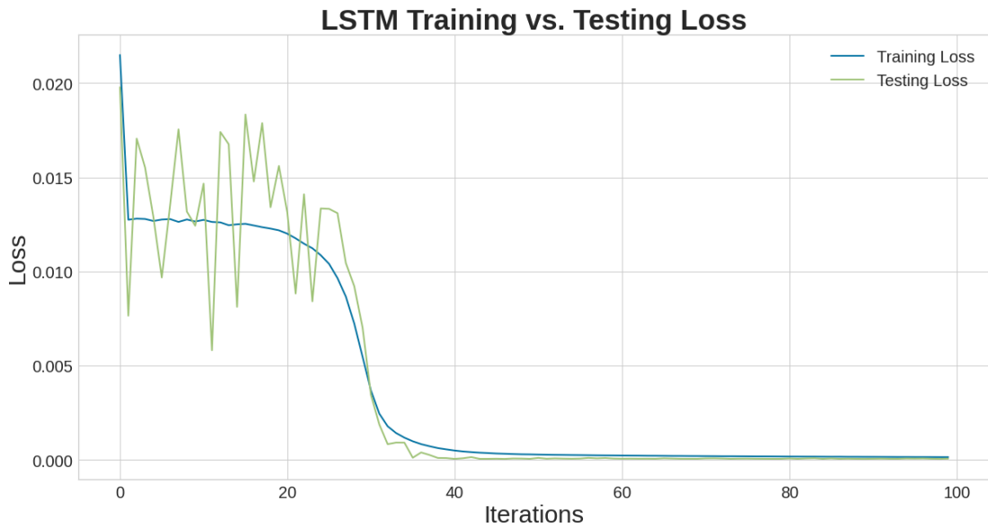
Figure 27. LSTM regression model training and testing loss plot, over the number of iterations.
