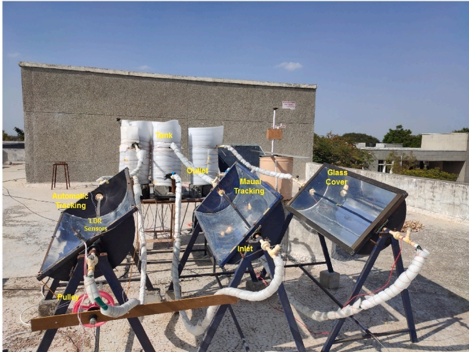
Fig. 5. Photograph of actual setup.
