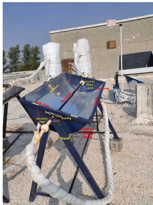
Fig. 3. Parts of PTC
