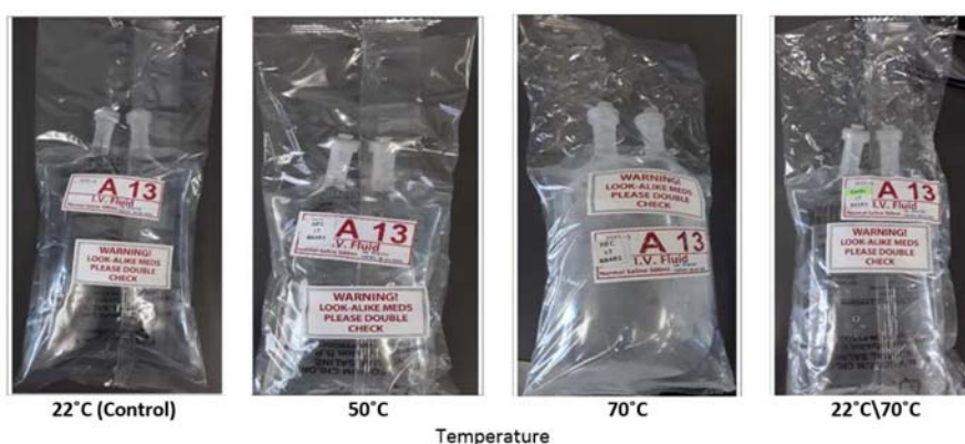
Figure 1. Influence of temperature on bulging of PO bags of normal saline after 28 days.
