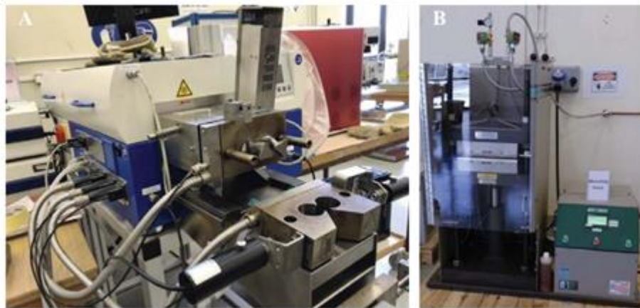
Figure 11:Plastograph internal mixer (A) and mounting press machine (B).
