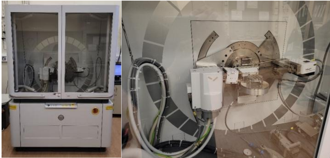
Figure 3-8. X-ray powder diffraction analysis setup at CAM.
