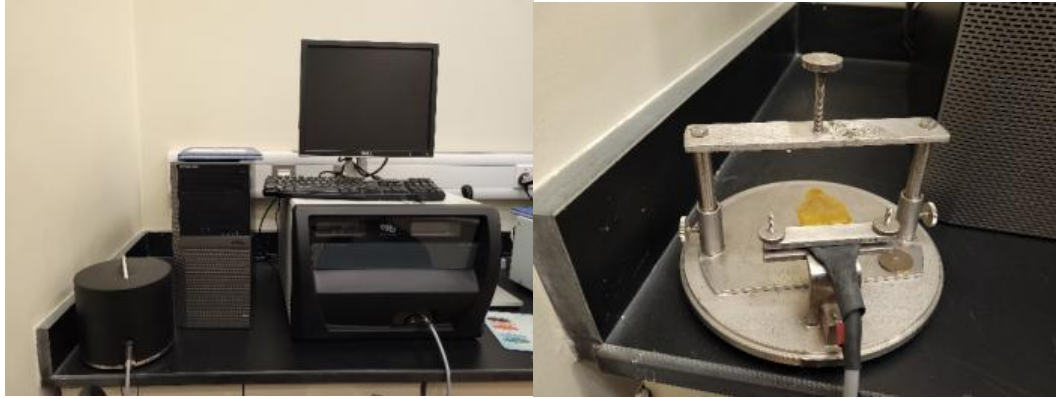
Figure 3-12. Hot Disk Thermal Constants Analyzer at CAM.
