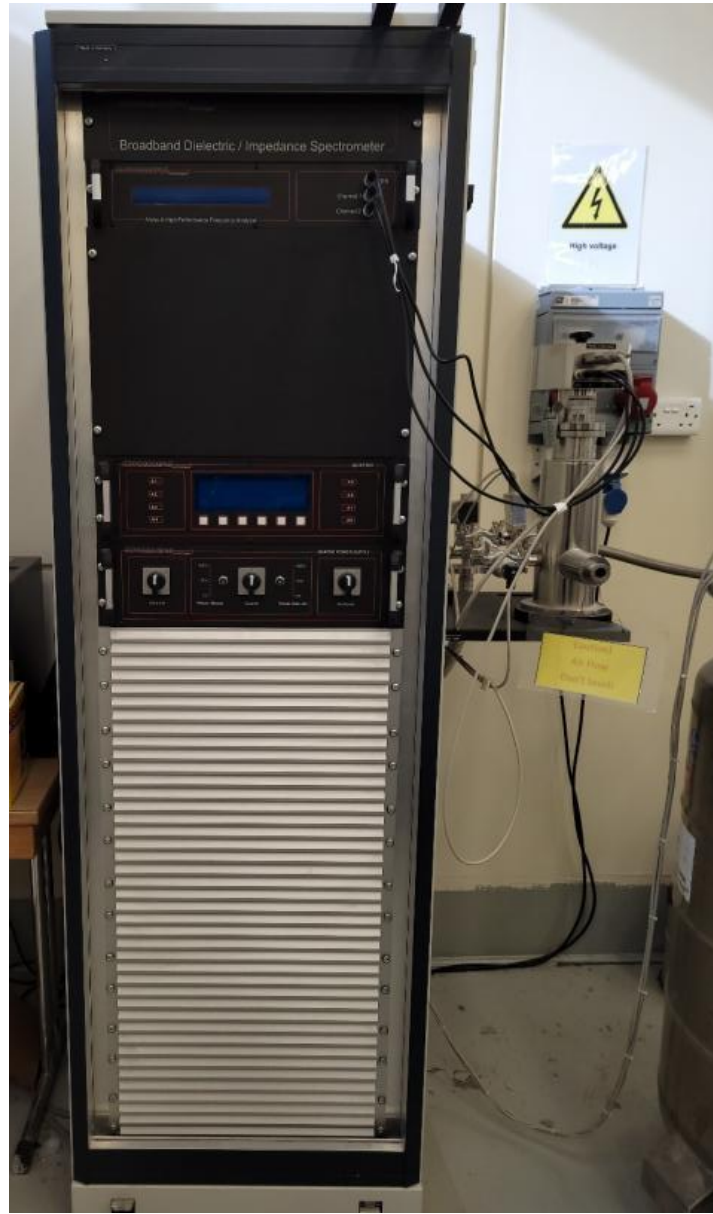
Figure 3-18. Broadband dielectric spectroscopy setup at CAM.
