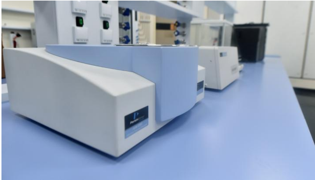
Figure 3-14. Differential scanning calorimeter setup at CLU.
