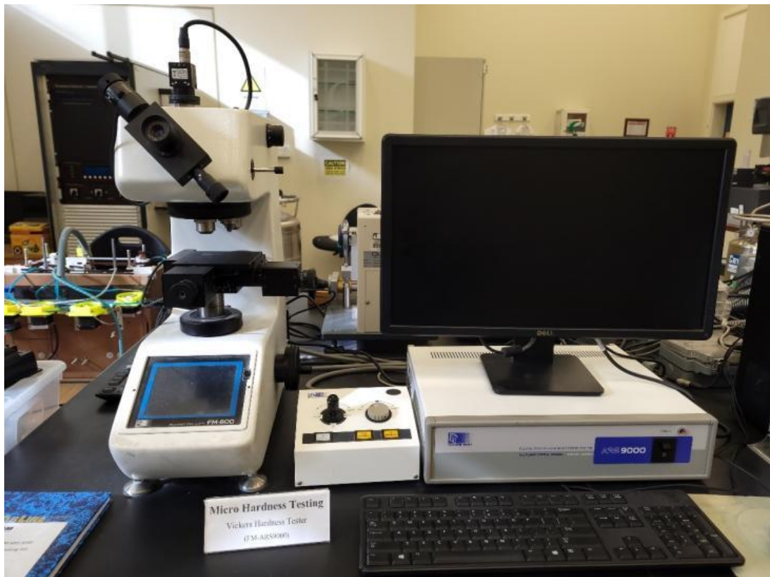
Figure 3-17. Microhardness testing setup at CAM.
