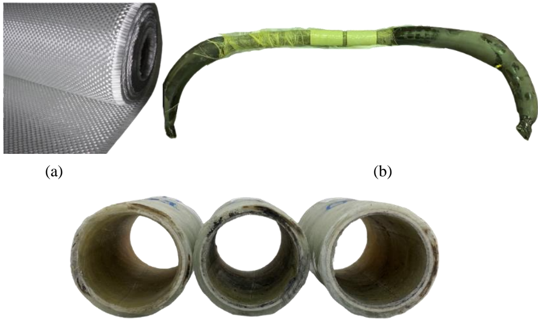
Figure 16. (a) Glass fiber fabric, (b) Inner wrapping process, (c) Internally and externally wrapped tubes
