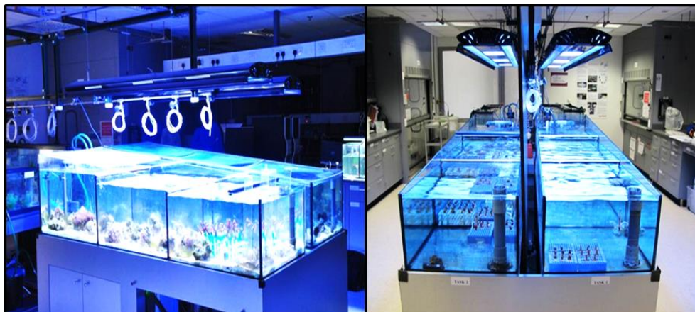
Figure 3. The setup of laboratory microcosms aquariums with controlled light, temperature and salinity
