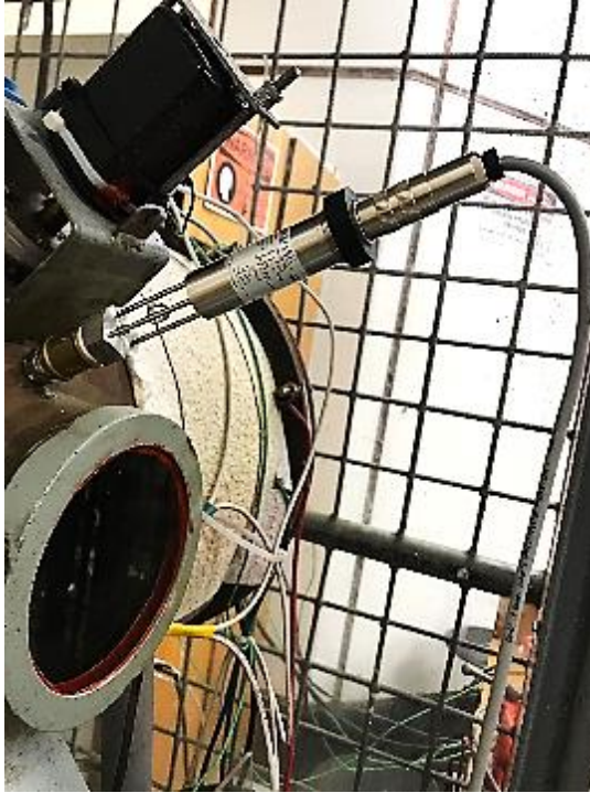
Figure 24. The pressure transducer mounted on the combustion bomb
