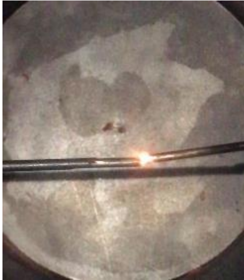
Figure 22. The spark produced between the two electrodes
