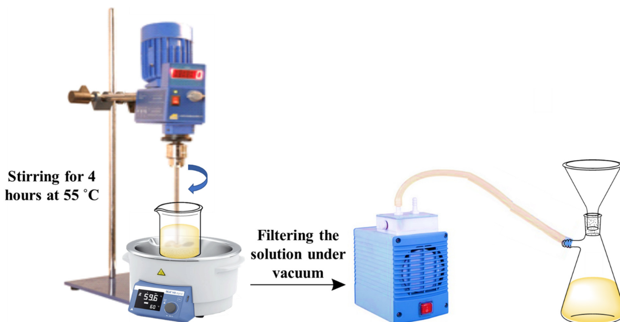
Figure 1. Schematic diagram illustrating the setup for the synthesis of urea-formaldehyde microcapsules (UFMCs) loaded with tung oil and linalyl acetate.
