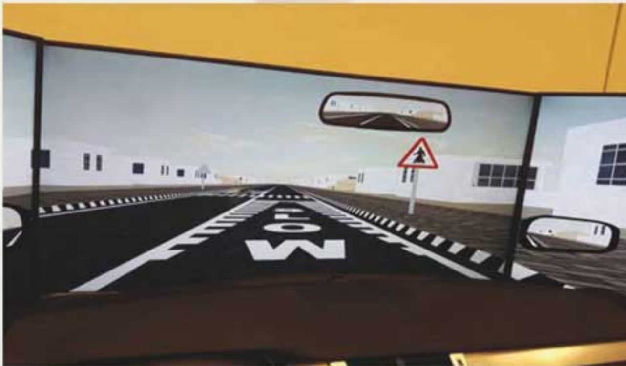
Figure 3. Pavement markings – Zigzag markings (left side), Road narrowing markings (right side).
