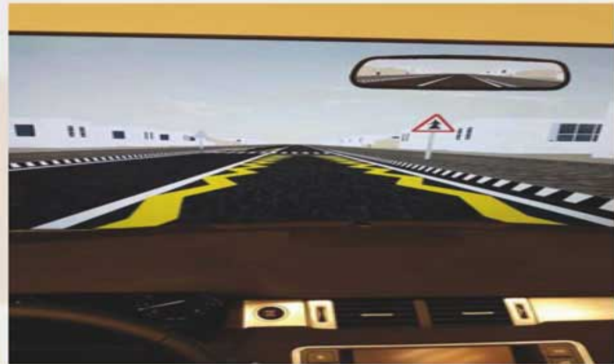
Figure 3. Pavement markings – Zigzag markings (left side), Road narrowing markings (right side).
