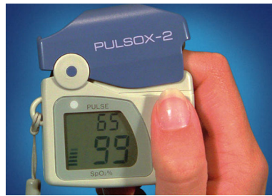
Fig. 8 A fingertip oximeter—a non-invasive but contact based method of measuring oxygen saturation by using a sensor placed on the fingertip. A variant of this technique is also becoming increasingly common in smartwatches such as devices from Fitbit and Garmin. Source: ©Teutotechnik, Med. Produktions- und Vertriebs-GmbH, Niedersachsenstr. 7,49186 Bad Iburg / Wikimedia Commons / CC-BY-SA-3.0 / GFDL
