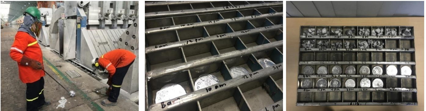
Figure 4.2: Bath and metal samples were taken and placed in proper place in able to be analyzed
