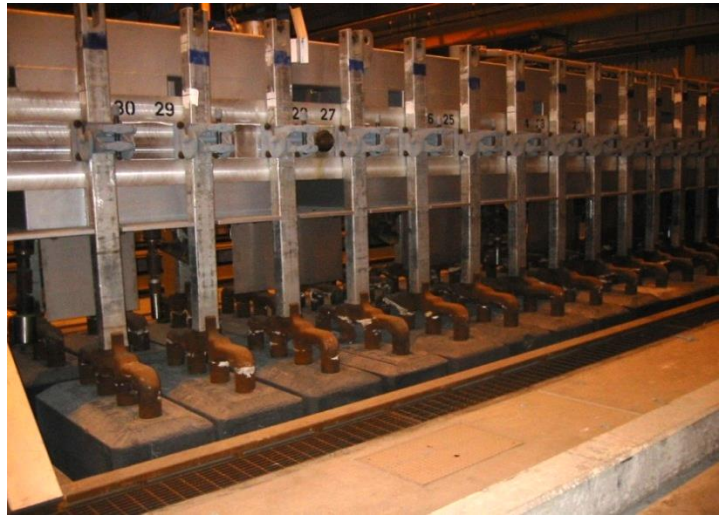
Figure 4.6: QATALUM side-by-side prebake cells with 30 anodes
