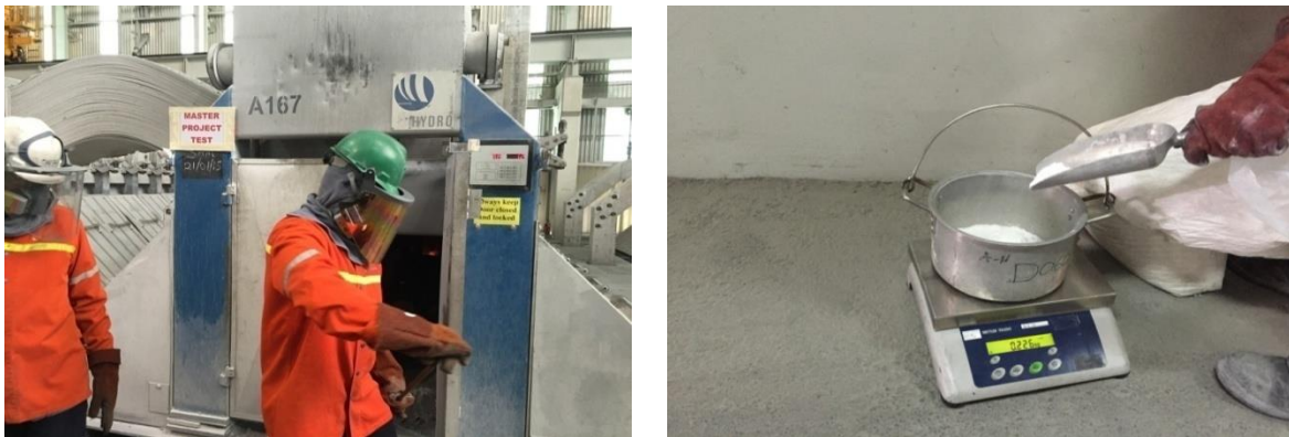
Figure 4.1: A certain amount of \text{Na}_3\text{PO}_4 , \text{AlPO}_4 and \text{SiO}_2 were added in the industrial cells
