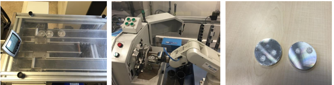
Figure 4.4: Metal samples were analyzed by automated optical emission spectroscopy (OES)
