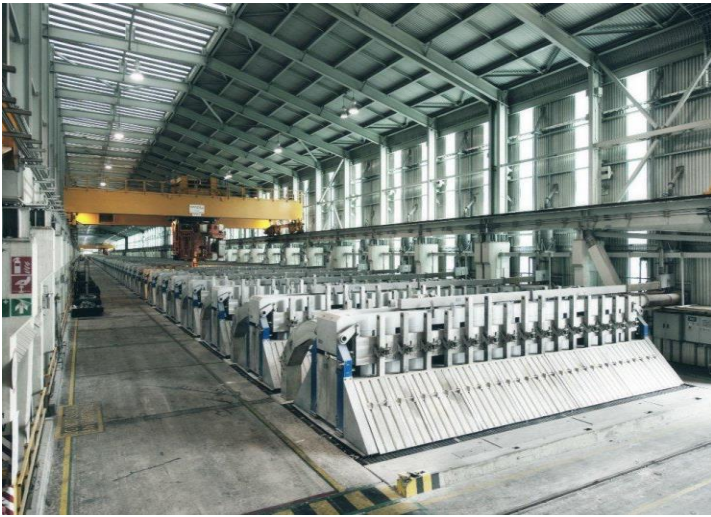
Figure 4.6: QATALUM side-by-side prebake cells with 30 anodes
