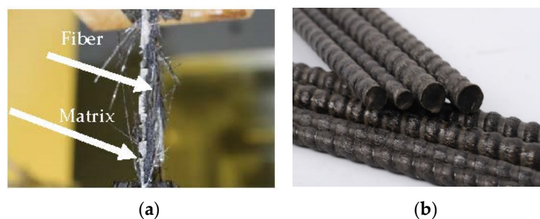
Figure 3. FRP materials: (a) FRP sheets (b) Basalt fiber bars.
