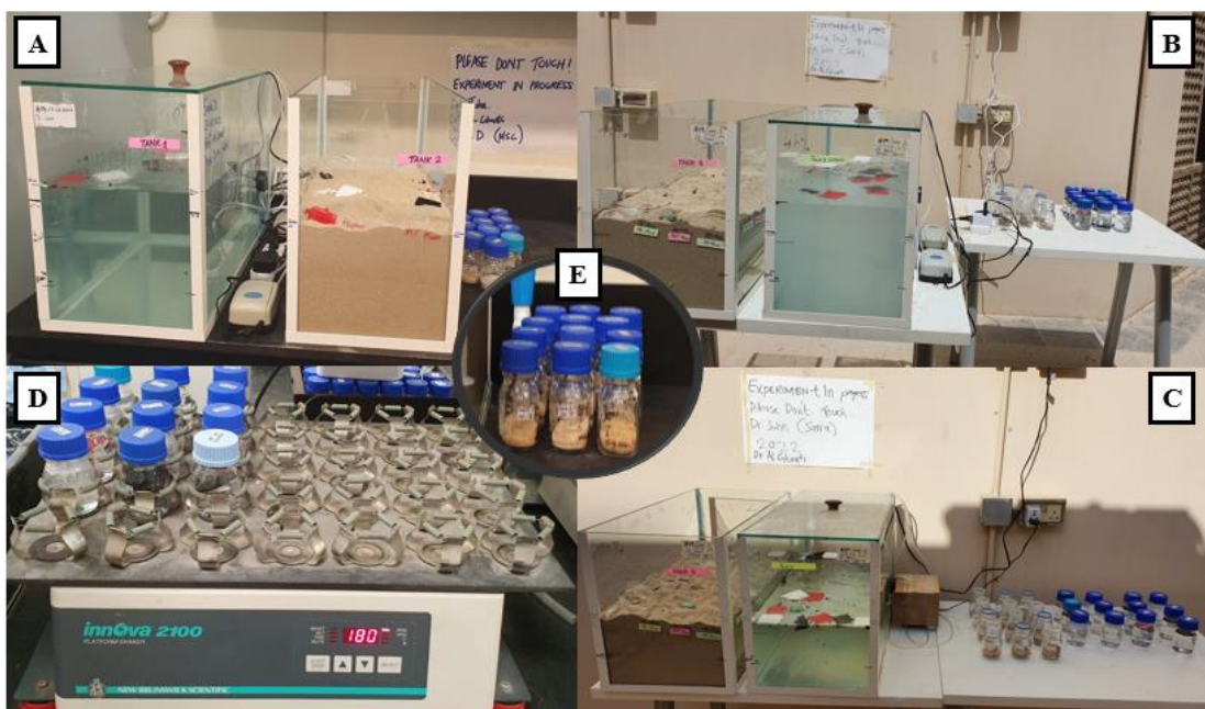
Figure 13. Indoor and Outdoor Experimental Set-up, A) Indoor Experimental Setup (T1 and T4), B) Outdoor Experimental Setup (Morning) (T2 and T3), C) Outdoor Experimental Setup (Afternoon) (T2 and T3), D) Small MPs Indoor Experimental Setup (Marine Litter Condition). E) Small MPs Indoor Experimental Setup (Onshore Litter Condition – T1 ).
