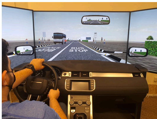
Fig. 1. Driving simulator: Qatar Transportation and Traffic Safety Centre (QTTSC), Qatar University.
