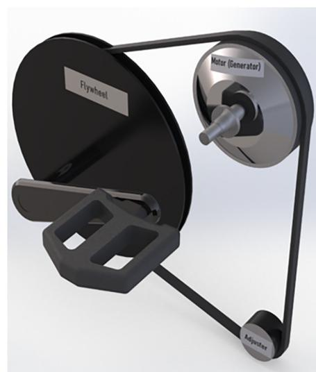
Fig. 5. Dynamo/flywheel connections.
