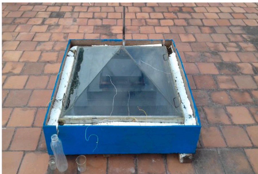
Fig. 16. Experimental setup of the multiple basin stepped pyramid solar still [100].
