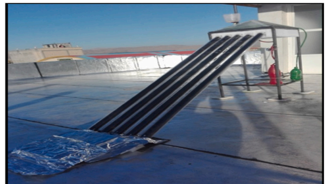
Fig. 4. Fabricated pyramid solar still with heat pipe collector [75].
