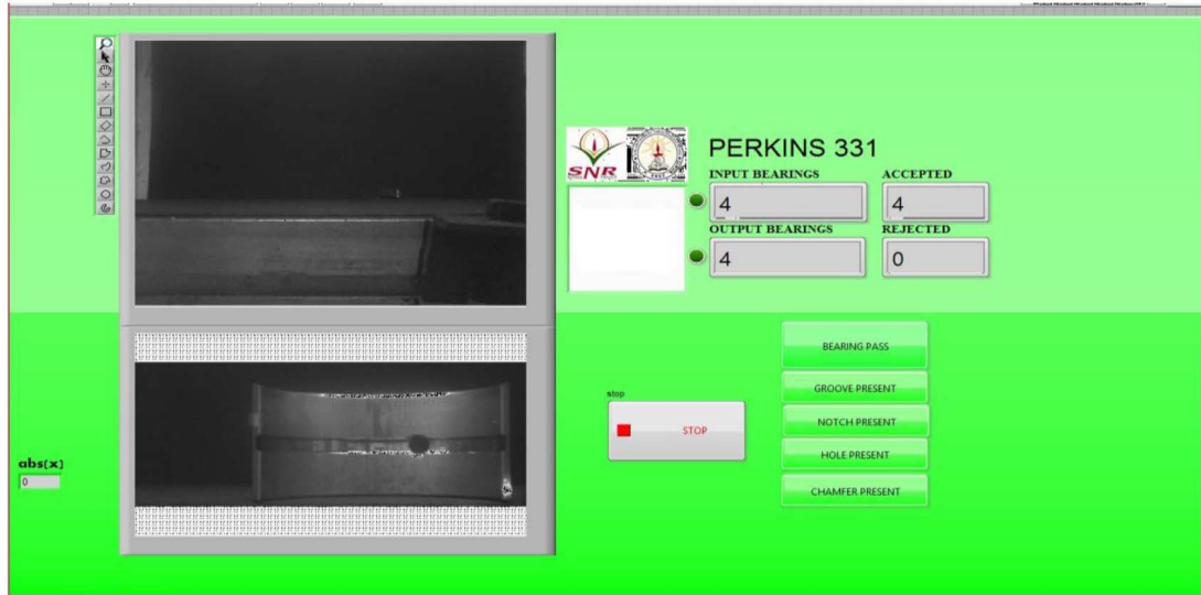
FIG. 4 Front panel of the automated system when the bearing is passed through the camera.
