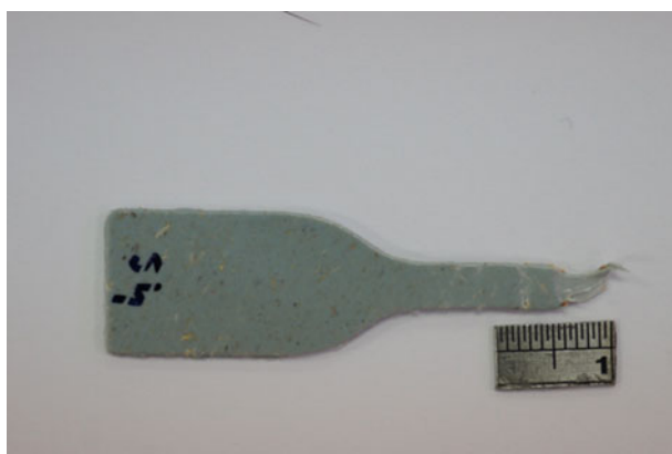
Figure 4 Tensile fracture sample of polyethylene (PE) composite made with recycled low-density polyethylene (LDPE) and wood as a filler
