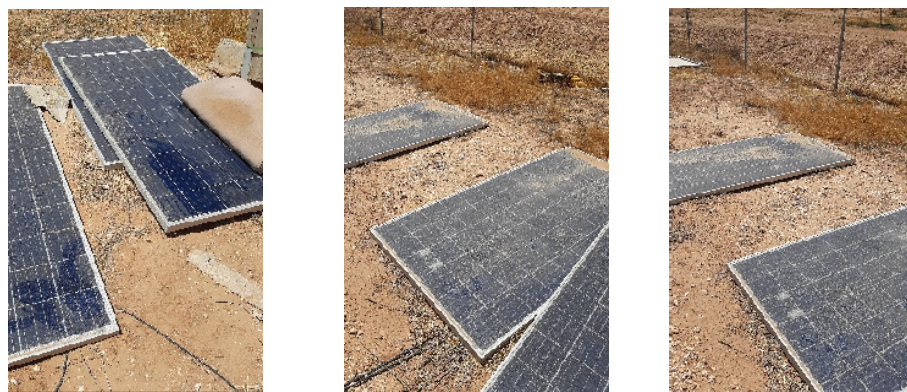
Figure 1. PV panels that are disposed of sporadically in the 3.2-megawatt capacity PV plant located in the north of Jordan (courtesy of Energy Department/Al-Albait University).
