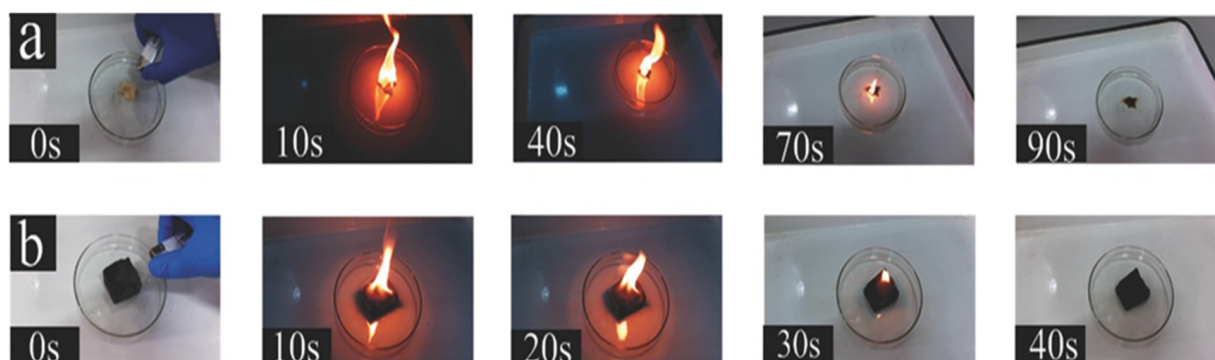
Figure 16. Video snapshots of the combustion of (a) MA and (b) rGO/MA containing adsorbed gasoline [107]; reproduced with permission from ELSIVIER.
