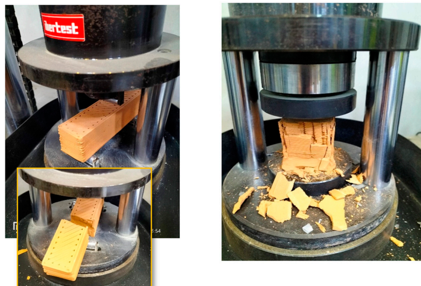
Figure 9. Printed Samples During Flexural and Compressive Strengths Testing.
