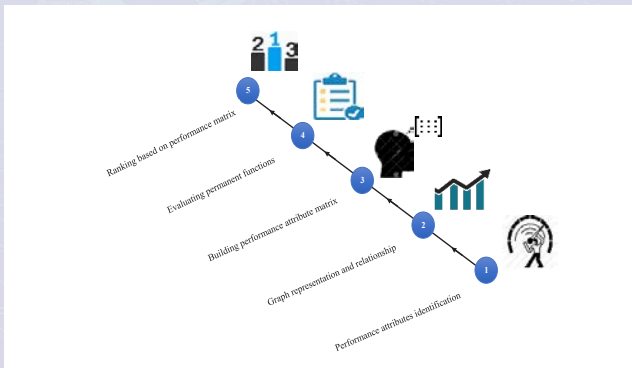
Figure 3. GTM approach step-wise procedure.
