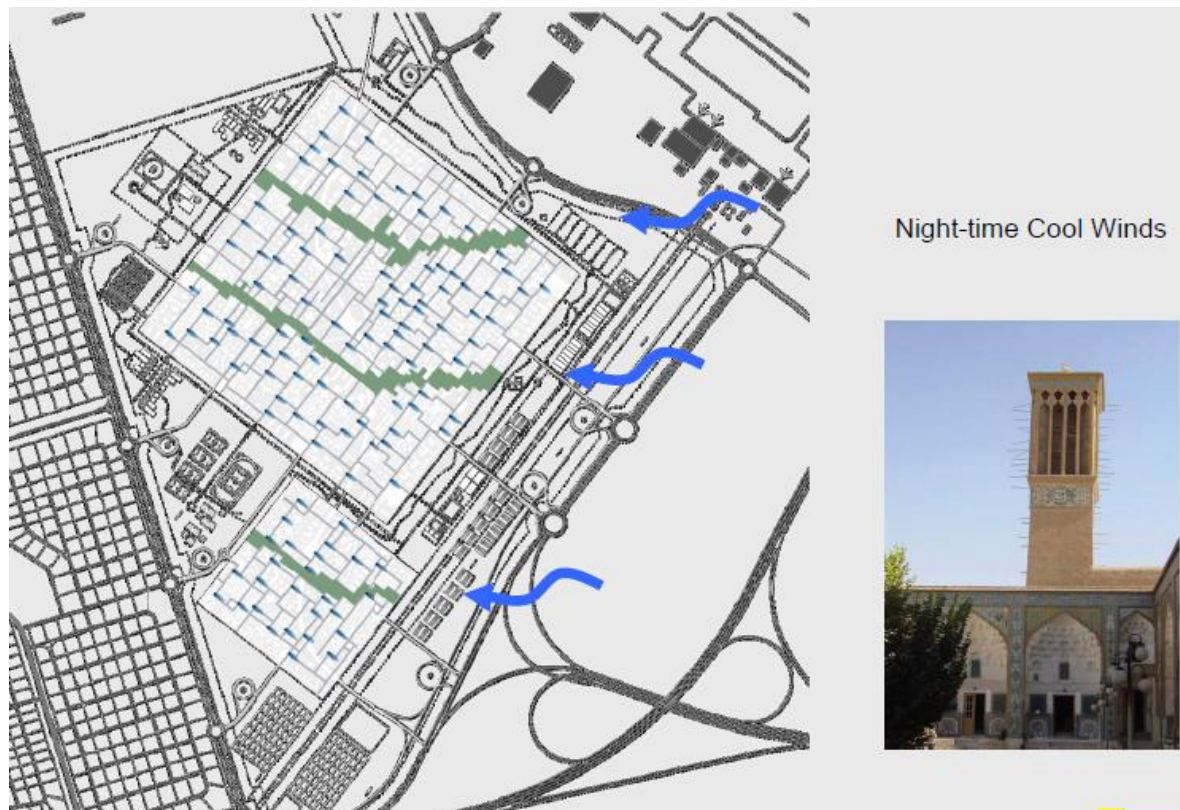
Figure 68: Wind Towers – Open, Cooling the Streets at Night by (Foster and Partners Architects, 2007)
