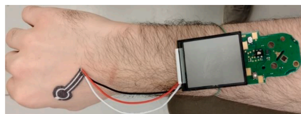
Fig. 13. Schematic representation of fabricated lactic acid detection.
