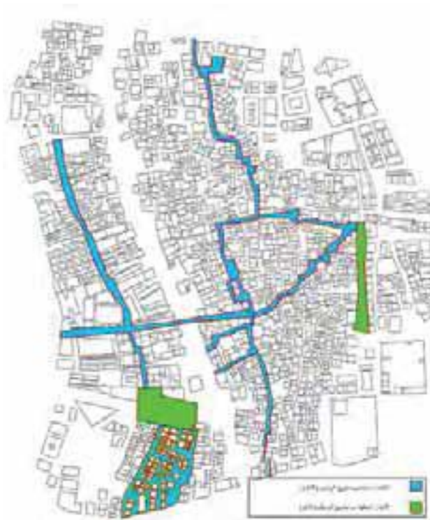
Figure 4-28. Repaved Streets in the Old City
