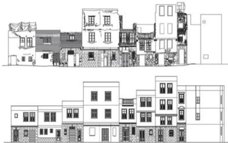
Figure 4-4: Houses in Afet Al Asaad Alley in Burg Al Zafaar Action Area – Before and After Rehabilitation (Source AKTC, 2007, pp.19)
