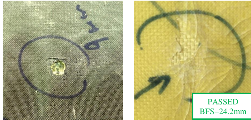
(f) Curved hybrid [CFRP 10 /KFRP 30 ] plate, sample #2, shot #1
