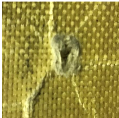
(a) Flat non-hybrid [KFRP 40 ] plate, sample #1, shot #1
