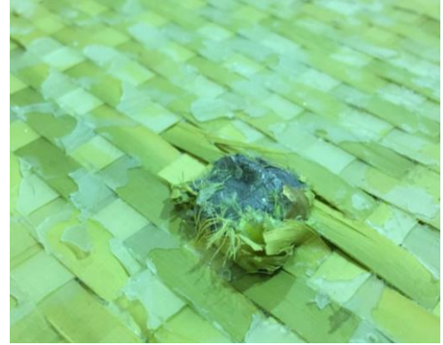
(b) Stopped bullet inside the [CFRP 4 /[DPRP 2 /KFRP 10 ] 3 ] plate
