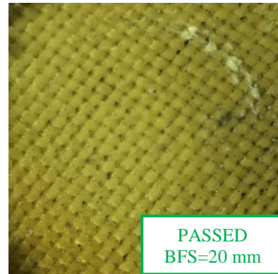
(a) Flat non-hybrid [KFRP 40 ] plate, sample #1, shot #1
