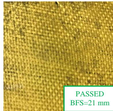
(b) Curved non-hybrid [KFRP 40 ] plate, sample #2, shot #1
