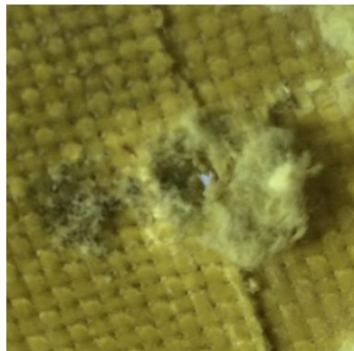
(b) Curved non-hybrid [KFRP 40 ] plate, sample #2, shot #1
