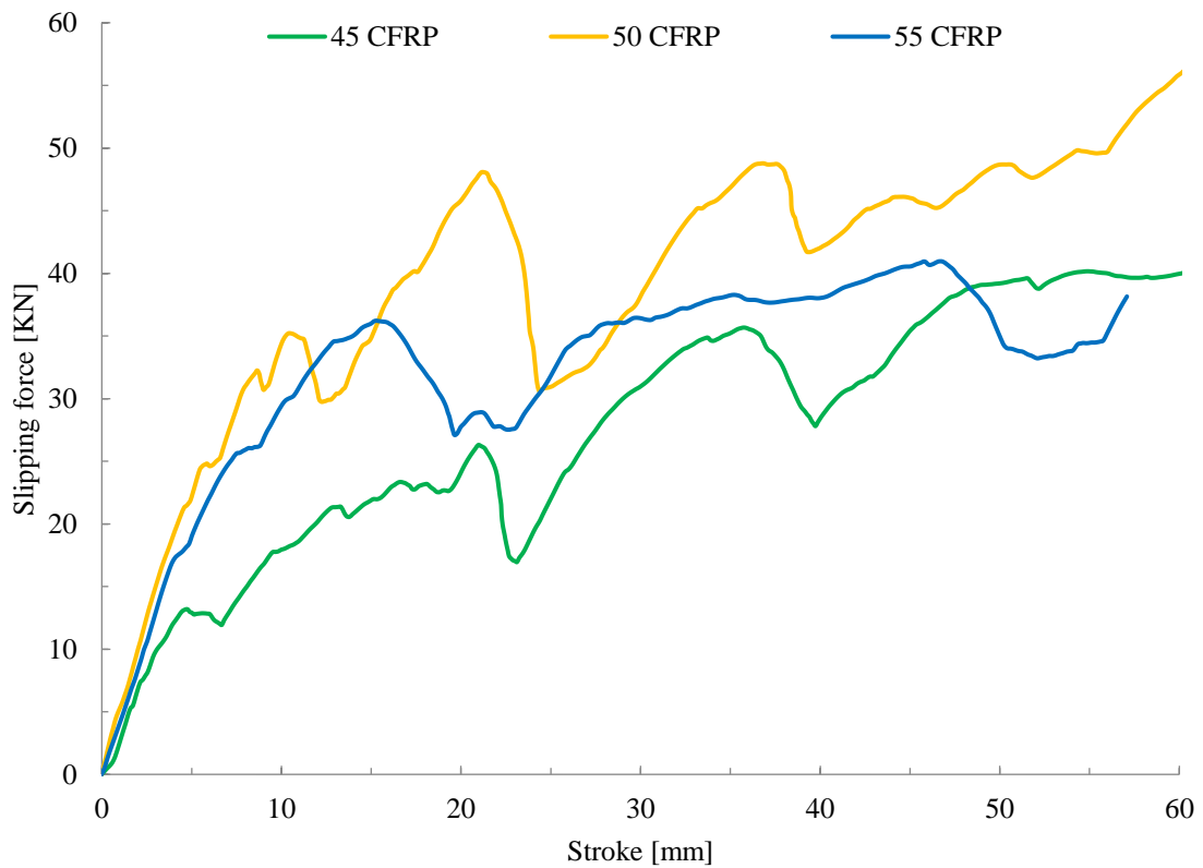
Figure 4-13: Experimental slipping force-stroke curve for SET-2 of the CFRP BGP
