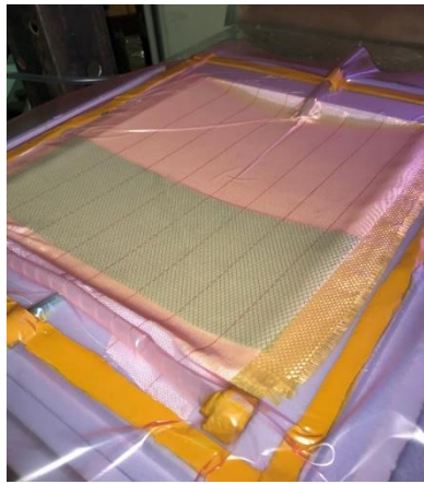
(a) Vacuum infusion fabrication process
