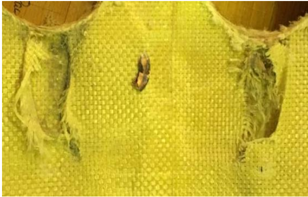
(a) Path of the stopped bullet in the non-hybrid [KFRP] 40 plate
