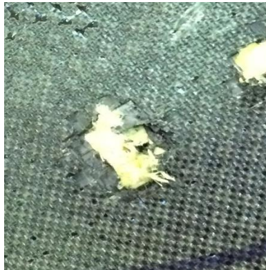
(d) Curved hybrid [CFRP 4 /KFRP 6 ] 4 plate, sample #3, shot #1
