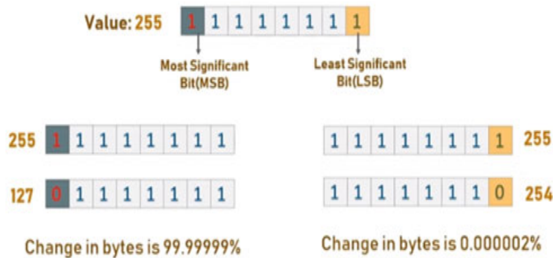
FIGURE 5. Explanation of the LSB (right) and the MSB (left) concepts.
