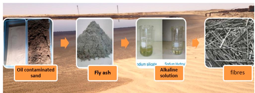
Figure 4. Materials used for mixture of oil contaminated sand, fly ash, alkaline solution and fibres.
