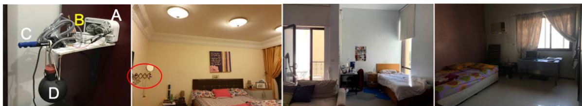
Figure 2. Instrument set-up and the survey environments (A: MX1102A; B: UX120-006M; C: hot-wire anemometer; D: Cu globe with thermal probe).
