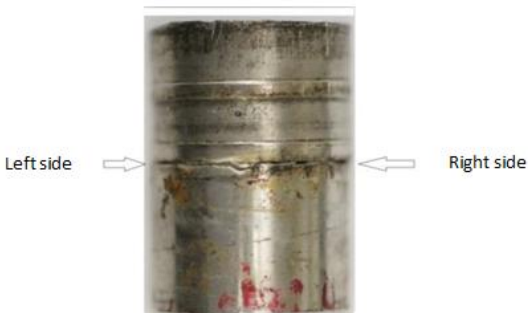
Figure 1. Overview of the as-received failed tube connected to the cooler pipe. Arrows refer to the inspected regions.
