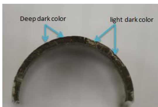
Figure 5. Overview of the fracture surface of 316L SS tube showing heavy oxidized regions (deep dark color) and less oxidized places (light color).
