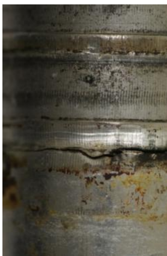
Figure 3. Photograph image for the crack region of 316L SS tube.
