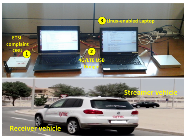
FIGURE 6. (Top) Table-top testbed setup with hardware components. (Bottom) Vehicles used in the field tests.
