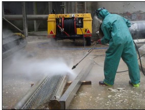
Figure 5: Water jetting machine [38]
