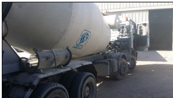
Figure 6: Ready mix Concrete (Transit Mixer)
