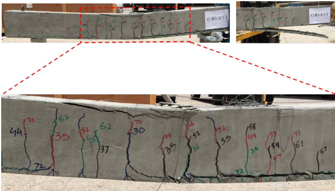
Figure 37: Mode of failure and crack patterns for test beam C-R1-V3-F (Values are in kN)
