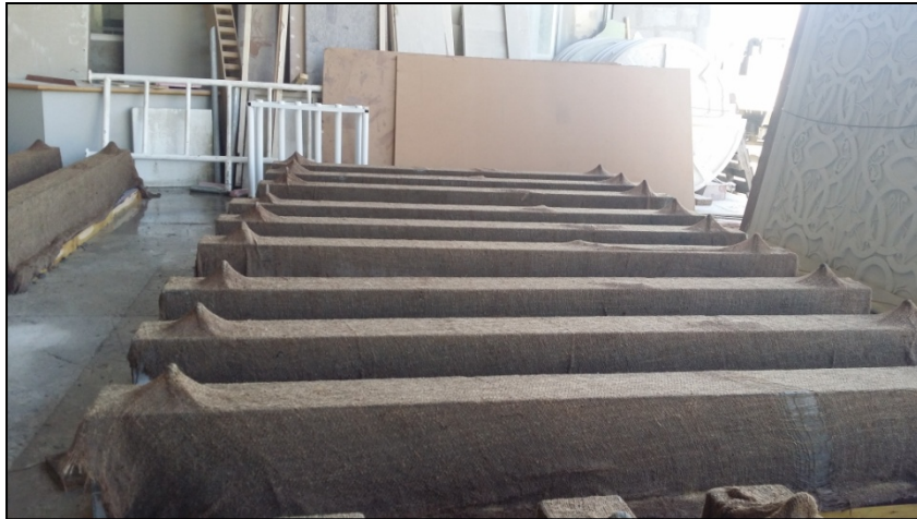
Figure 18: Curing of beam specimens
