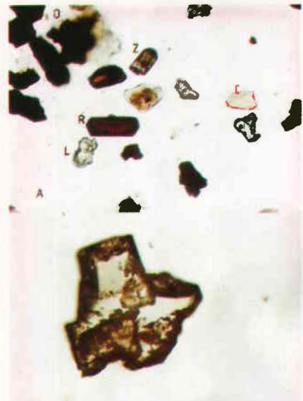
Figure (6): (A) Rutile, euhedral prismatic, dark red grain (R); Leucoxene (L); Opagues "mainly hematite" (O); Zircon (Z); Clinozoisite (C), depth 930 meters. Ordinary light, X10.
