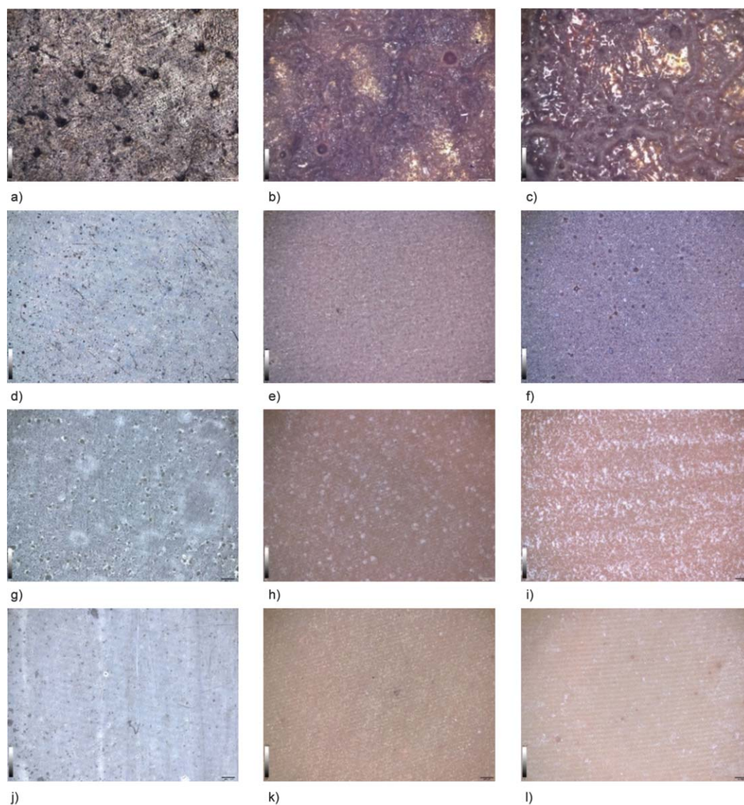
Figure 3. Bright field optical images of control epoxy coating at a) 0 day, b) 30 day, c) 45 day of exposure; EP/HNT/Imeso; d) 0 day, e) 30 day, f) 45 day of exposure; EP/TNT1; g) 0 day, h) 30 day, i) 45 day of exposure; EP/TNT2; j) 0 day, k) 30 day, l) 45 day of exposure
